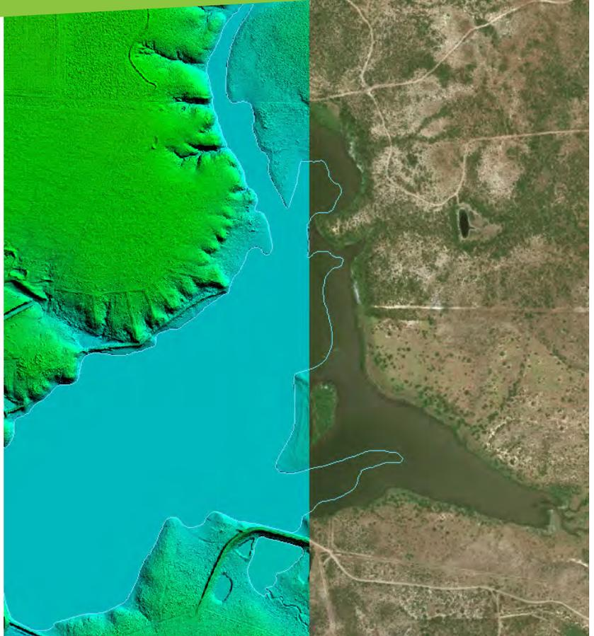
**Hydrological feature from project lidar data (left) compared to non-drought imagery (right)**
